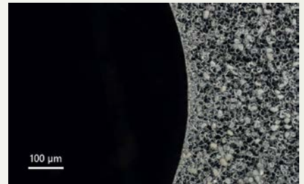
SEM image of processed FZ-Si wafer edge. Courtesy of FTMC.
