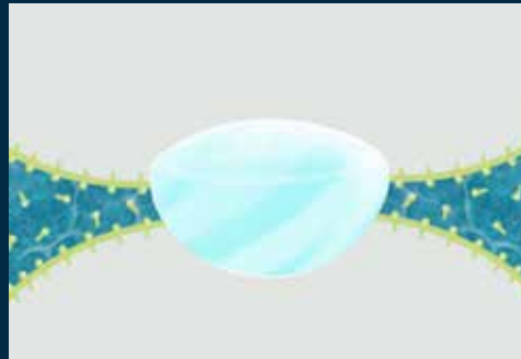
Figure 2: Dewetting of the defoamer drop.
