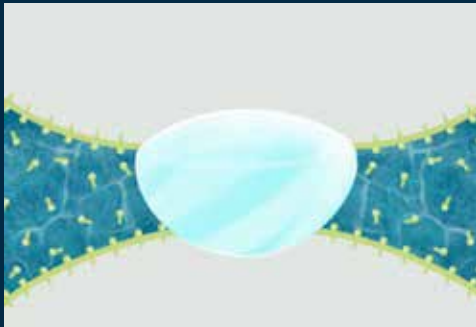
Figure 1 (Bridging Mechanism): Defoamer drop breaks through the foam lamella on both sides.
