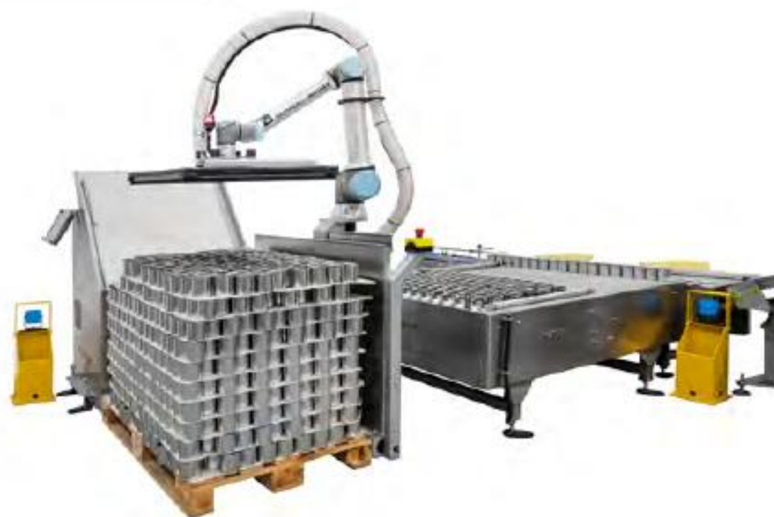
Pail Denester PAILMANAGER-V-FLEX ● From 12 to 22 pails/min
