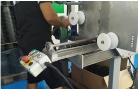
Hose winder station
